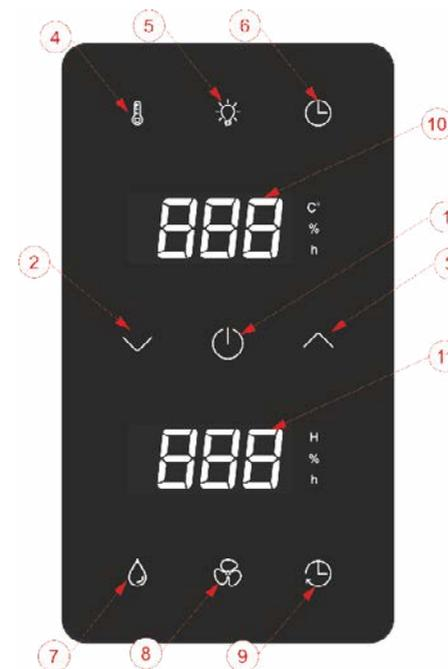
Fig. 10 Control operating elements
