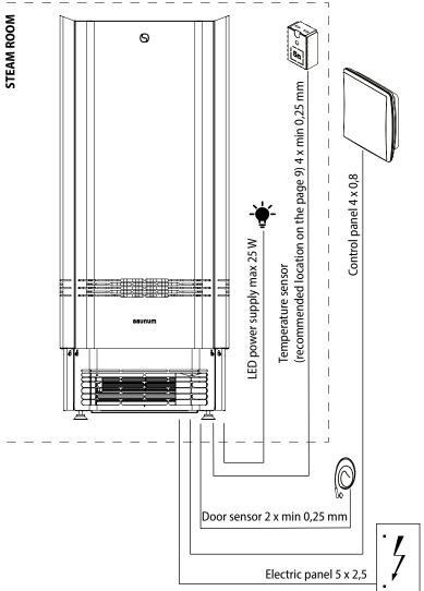
NB! Due to the potential danger of thermal embrittlement, it is forbidden to use a PVC-insulated cable as the connection cable for the sauna climate device.
