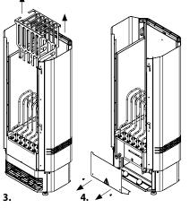
**4.** Remove the panel covering access to the heating elements. Undo the two bolts holding it in place
