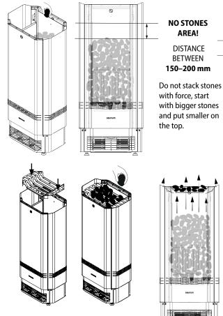
When you have filled the basket with stones like shown in graph, reposition the top grille and then add stones to it on and ensure that the air can move freely. Do not pile up and stack rocks on top of each other.
