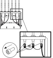
5. Release all the heating element cables.
