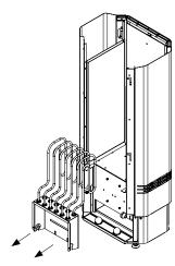
**6.** Undo the bolts holding the heating element module in place.
