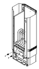
7. Remove the heating element module.
