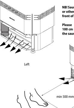
NB! Sauna users must not keep their feet or other body parts closer than 50 cm in front of the working fan!
