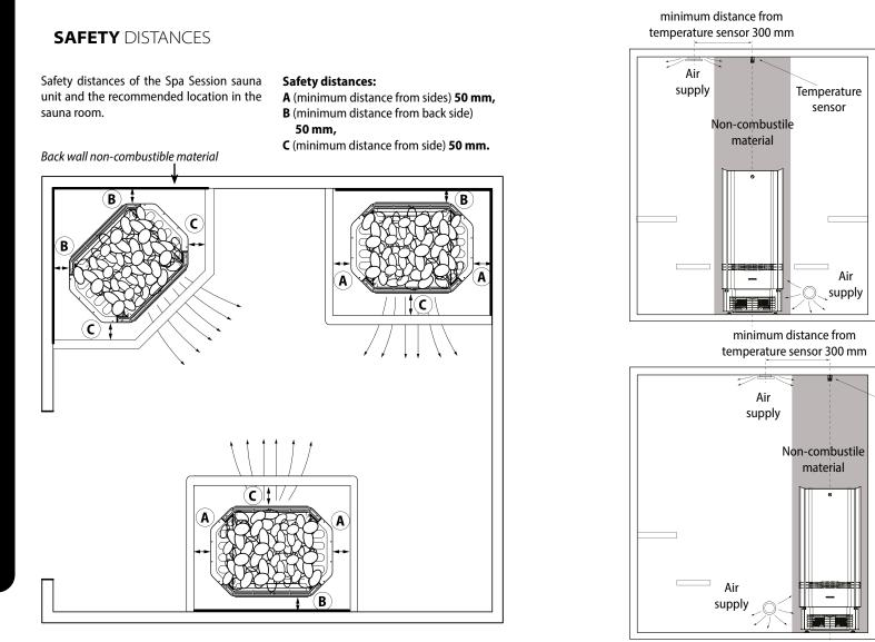
minimum distance from temperature sensor 300 mm
