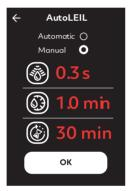
The exact amount of water dispensed depends on the water tap pressure. Please note that, in most cases, with good water pressure a 2–4 second value for water quantity can be an excessive amount of water. We recommend to start testing with 0.5–0.8 seconds to get a feel.
