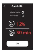
The maximum relative humidity value that can be applied in Automatic Mode is correlated to the previously set temperature value. For example, it is not possible to set a more than 30% RH in a 70C sauna. The approximate temperature/humidity limits are shown on the graph below.
